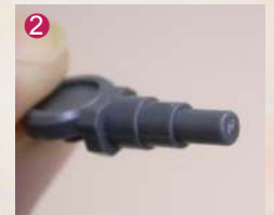
▲ If the gate is at the corner of a part, you may accidentally cut off some of the part along with it. The photo shows an example of this kind of mistake. You have to place the nippers at an appropriate angle to prevent cutting the piece along with the gate.
