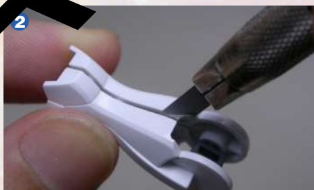
▲ Gradually you are going to see a gap opening up between the parts. Change the position of the knife and repeat the process until there is a gap between all the joints. If you can remove the parts evenly, they won't be distorted, and you can assemble them again later.
