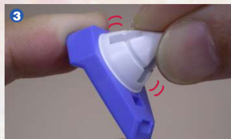
▲ If you don't have enough room to insert the blade between parts, try to move them little by little so that they come loose. Repeat this several times, and they will gradually come off.
