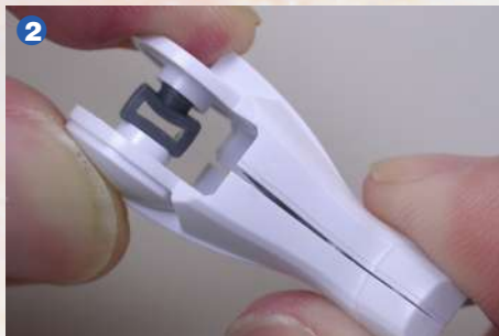
▲ This is a bad example of installing a polycap. If it's not properly inserted into its socket, the peg will be crushed. A polycap with a hole easily warps when pressed.
