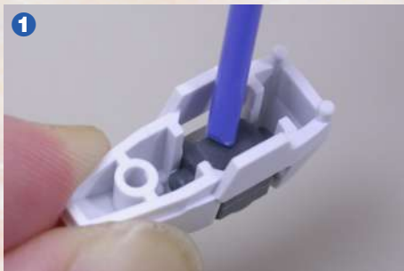
▲ Here I am inserting a polycap into a part. It is difficult to push it in with fingers, so I used a stick (in this case, a cut off from a runner). You should adjust the orientation of the polycap so that it will not tilt inside.
