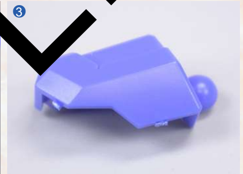
▲ The part detached from the runner. You can see that the cut end of the gate is jagged. If you forcefully try to cut the edge of this area, the rough area may get bigger.
