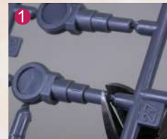
▲ If the gate is at the corner of a part, you may accidentally cut off some of the part along with it. The photo shows an example of this kind of mistake. You have to place the nippers at an appropriate angle to prevent cutting the piece along with the gate.
