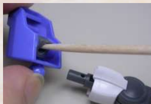
▲ Place the tip of a knife between the parts where they join, then twist the knife a little to make a gap between them. The parts can get scratched, so it is better to place your knife's tip where the scratch will not stand out.
