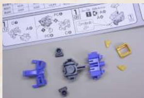
▲ Let's assemble the part from the first example. First, connect to one side the polyethylene parts that will need to be sandwiched together. Next, align both parts along the direction of the pegs (horizontal in this case). Be careful not to tilt them.
