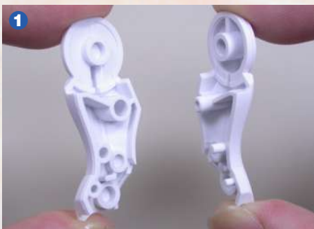
▲ An example of snap-fitting. You can secure parts by connecting the pegs on their back to the corresponding holes. If the peg is long or if there are multiple pegs on the same part, it means that it will be secured more tightly. Pegs may also be flat like plates.
