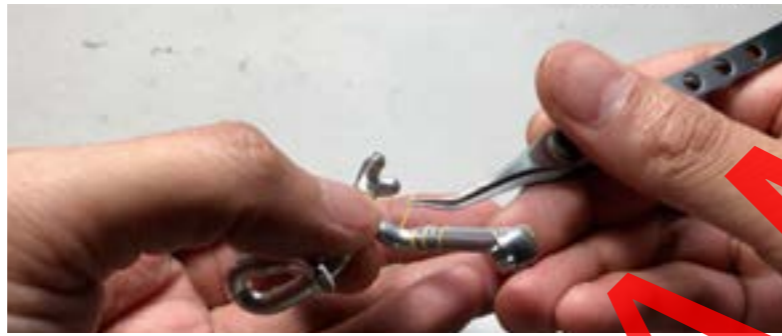
I painted muffer components silver. Then, I applied thin strips of masking tape, mainly along the exhaust joints.
