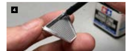
The integrated radiator was separated to better suit the naked design. I roughly cut it with nippers, then refined it with a file, and painted the edges silver (1 - 3). I left the fin section unpainted and finished it with panel lining (4).
