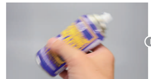
▲ Before using a spray can, vigorously shake it to ensure the paint is well-mixed. Metallic colors, especially, have heavier particles that can settle easily. Shaking the can approximately 100 times will help ensure an even paint mixture.
