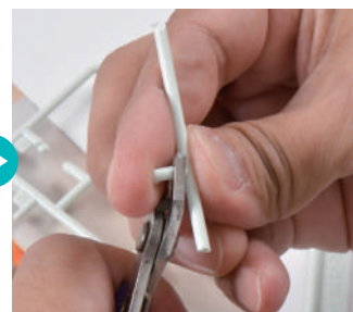
▲ First, pick out a runner that you want to use for extra detail on your gunpla. Grab your runner nippers (they are quite affordable and available at most hobby stores) and carefully cut away the nubs. Try to choose sections with fewer nubs – it is easier to turn such a runner into a simple rod shape.
