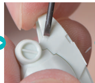
▲ I also added a V-shaped line detail using a chisel, starting from the edge on a short line.
