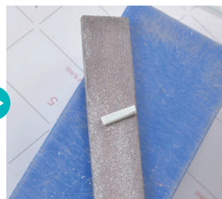
▲ Now for the fine-tuning. Cut the plastic to the desired size, then use a hand file to slowly and carefully shave it down to the desired thickness.
