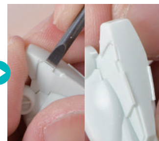
▲ I decided to carve a line above the detail. I'm going to carve a V-shaped detail with a chisel that's wide enough for the line I want to engrave.
