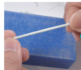
▲ Use a hobby or craft knife. Gently shave down the plastic until it's flat.
