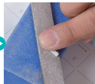
▲ Here's a simple technique for controlling thickness: Place the runner flat on a metal hand file. Use your fingertip to gently press down on the runner and move it to shave off small sections.
