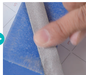
▲ Here's a simple technique for controlling thickness: Place the runner flat on a metal hand file. Use your fingertip to gently press down on the runner and move it to shave off small sections.
