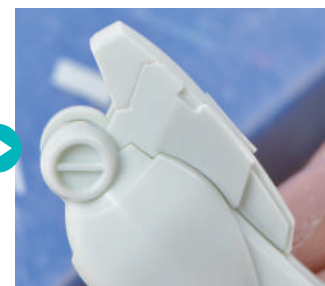
▲ The finished engraving line details on the side of the knee armor.
